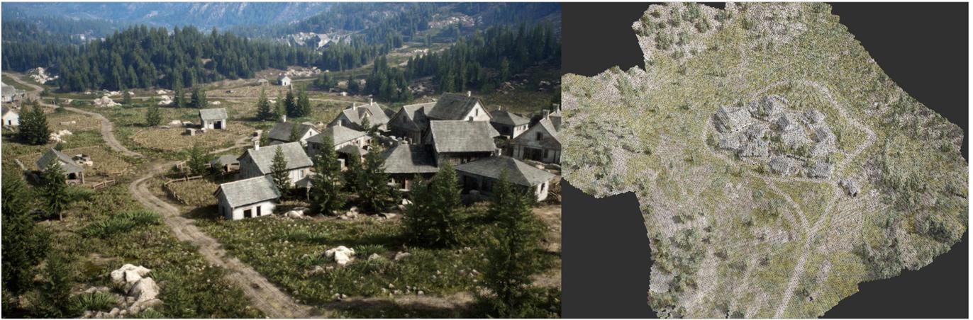
Fig. 2. The (left) Mountain Grassland Environment used and (right) extracted SIM gold-standard (“truth”) in UFOMap at 1m resolution.
